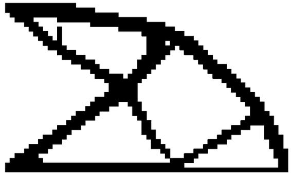
Fig. 7. The result of the cantilever beam example after the trivial solid filter.
